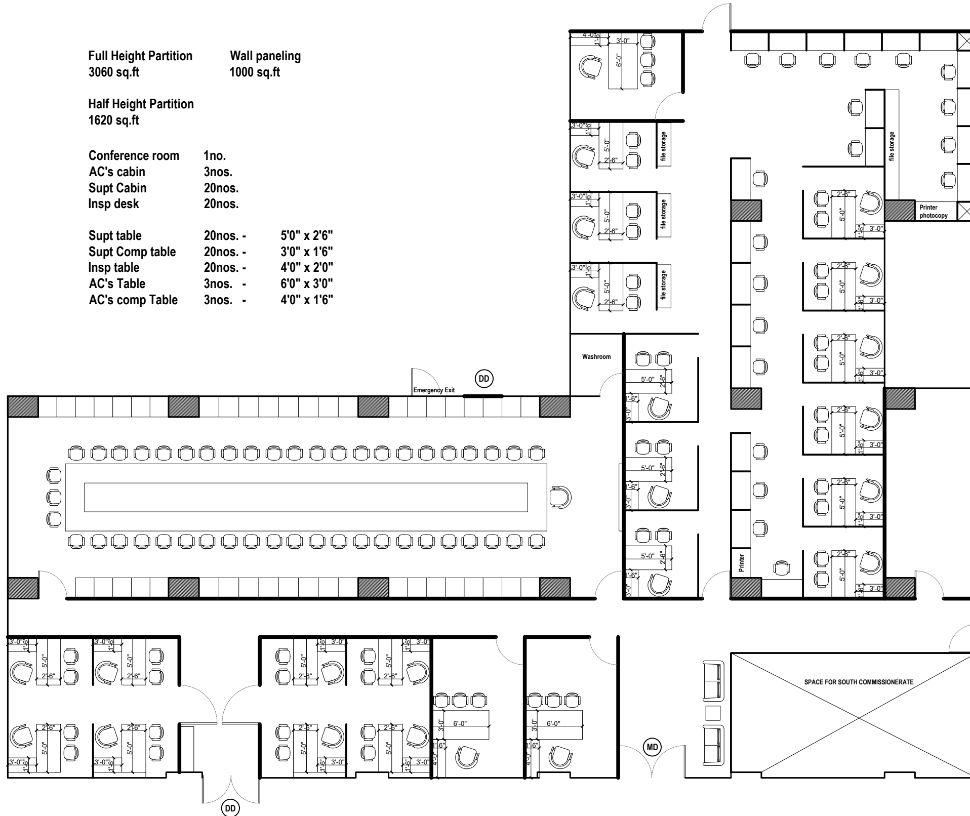
PROPOSED INTERIOR LAYOUT FOR GST AUDIT AT FOURTH FLOOR NORTH WING , MHU COMPLEX , NANDANAM AREA : 4850 Sq ft.
